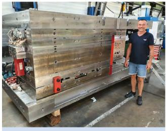
Installing the 4-cavity mould.
