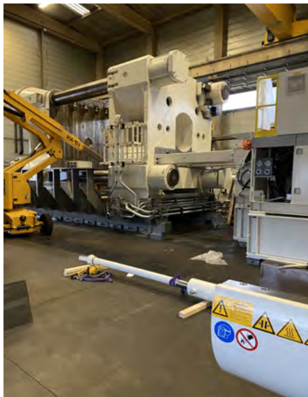
After several weeks of assembly, the new 6000-tonne injection press is finally operational.
