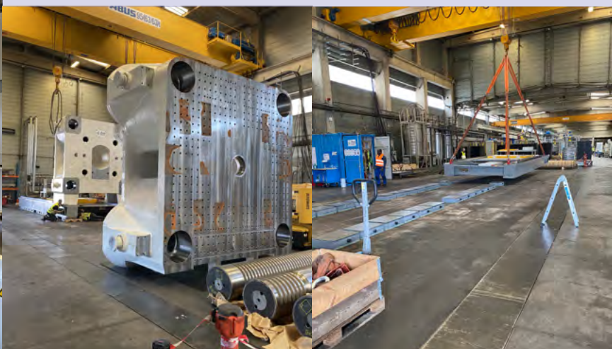
After several weeks of assembly, the new 6000-tonne injection press is finally operational.
