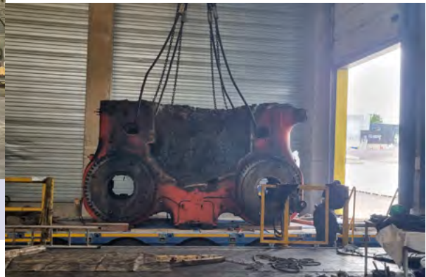
After several weeks of assembly, the new 6000-tonne injection press is finally operational.
