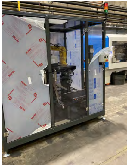
New bagger allowing us to bag all small elements.
